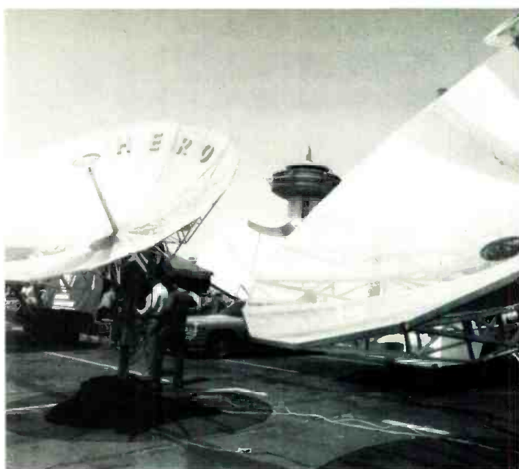
Hero Communications' Super Tennas are aluminum mesh transportables which come in five sizes, from three to 7.56 meters.
