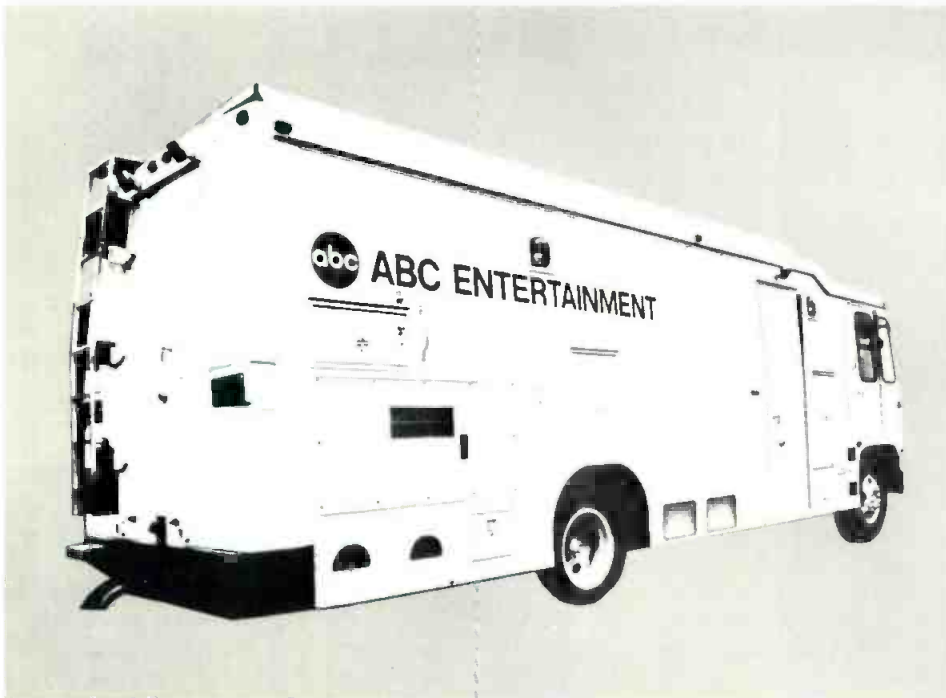
A.F. Associates recently completed this 29-foot mobile unit for ABC-TV. The van includes two Ampex one-inch VTRs, GVG switcher, and Yamaha console.
